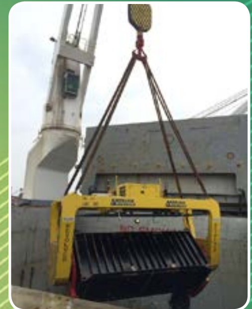
Containers being tipped into ships hull.
