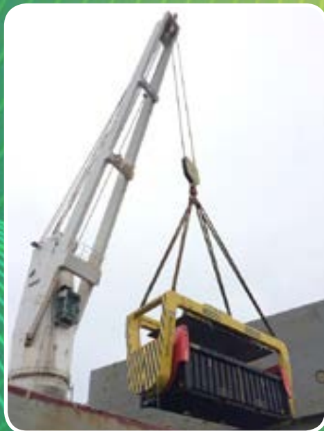
Patented lid lifter replacing the container lids.
