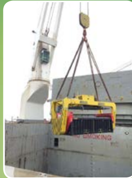
Patented lid lifter in use.
